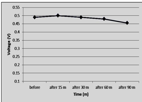
Figure (7): Open circuit voltage with a time of laser irradiation for solar cells sample
