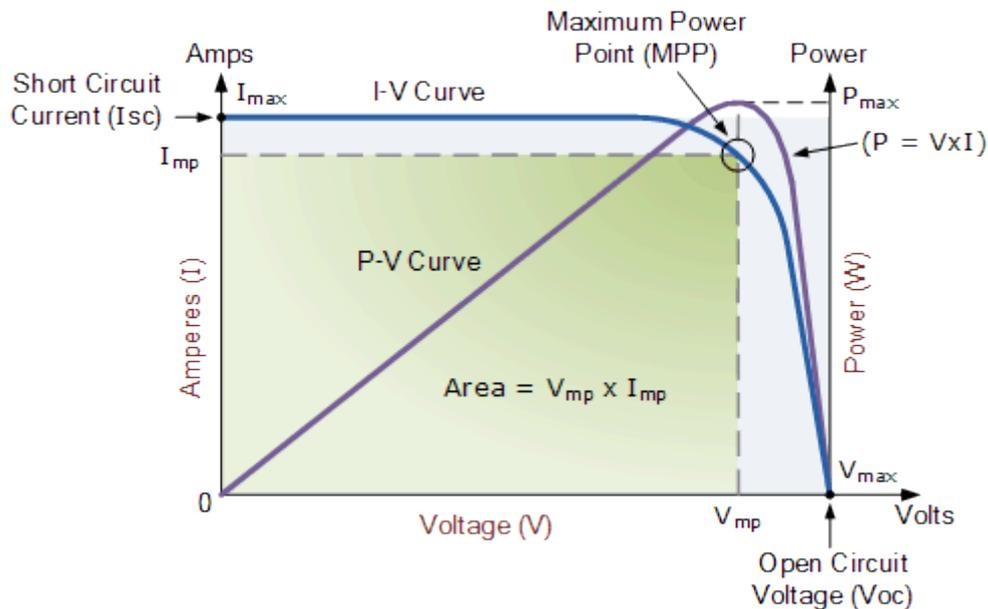
Figure (1) : Characteristic curve of the solar cell[11]
