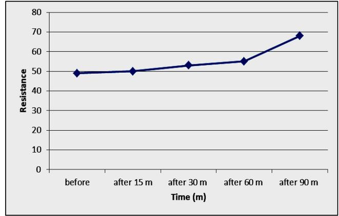
Figure (12): Shunt resistance with a time of laser irradiation for the solar cell sample
