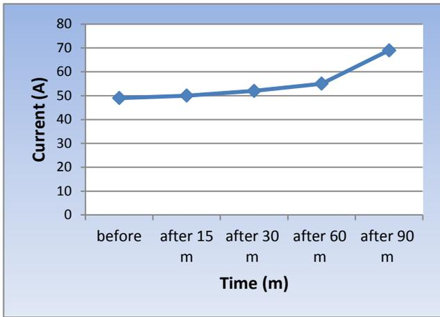
Figure (6): Short circuit current with the time of laser irradiation for the solar cell sample
