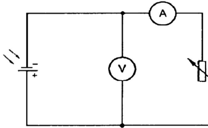
Figure (4) : Circuit for I-V characteristics of solar cell
