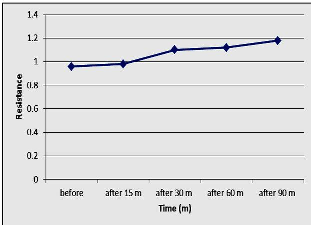
Figure (11) : Series resistance with a time of laser irradiation for solar cell sample
